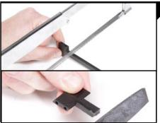
Using a hacksaw with a wood or metal blade cut all they way through the marked line on the spacer. After cutting the spacer to the appropriate size use a file to smooth off any loose material as seen in Figure
