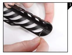
While holding onto the sight, flip the heatshield over and using the provided 4-40 x 3/8" flat head socket cap screw and a 1/16" allen driver, tighten to the heatshield as seen in Figure 3.
