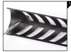
While holding the rear ghost ring sight in place, turn the heatshield over and insert the provided 4-40 x 3/16 " phillips head screw into the base of the rear ghost ring sight. Using a small phillips head screwdriver tighen the screws as seen in Figure
